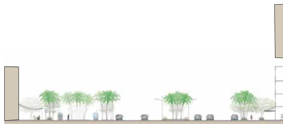
Illustrative arterial boulevard street section.
