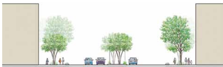
Illustrative arterial boulevard street section.
