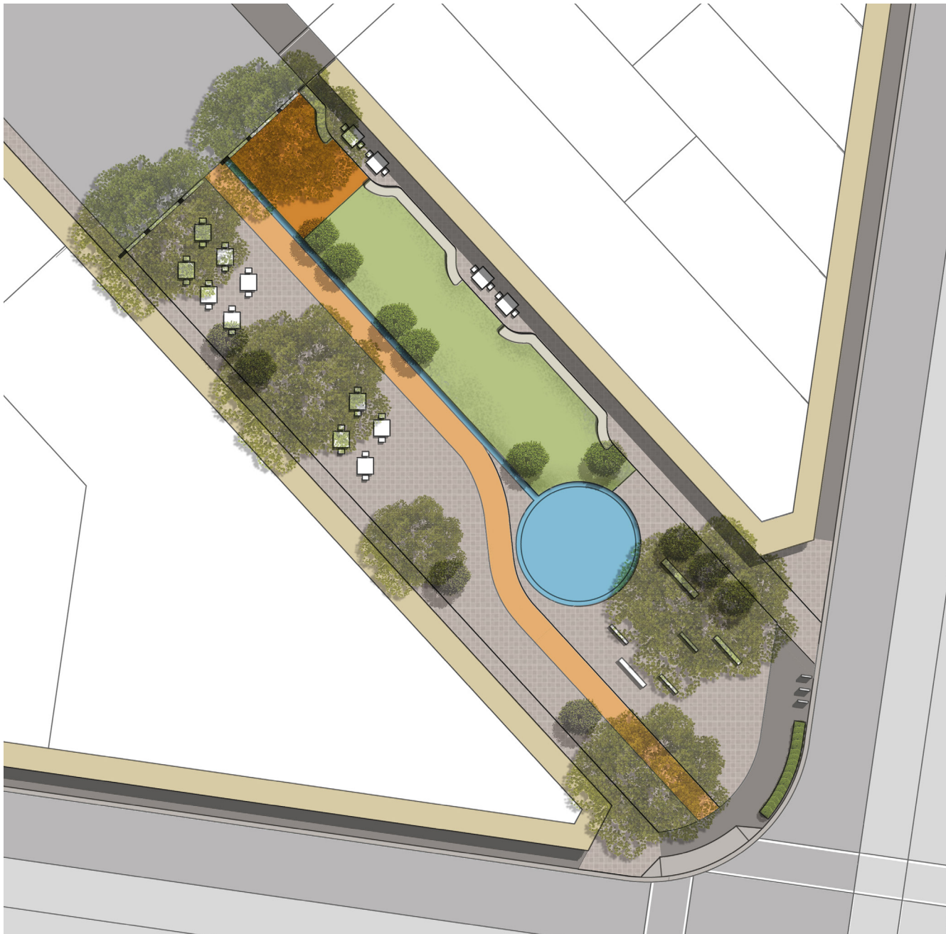
Figure 16: Indicative design of the northern plaza, showing a gathering area, alfresco dining, cycle path, planning and playground.
