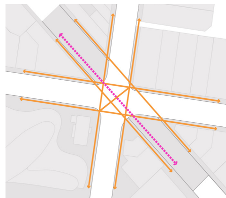
Figure 13: Any reconfiguration of the Junction should facilitate easy movement of pedestrians and cyclists. Pedestrian desire lines are shown in orange, Camberwell road cycle movement in magenta.
