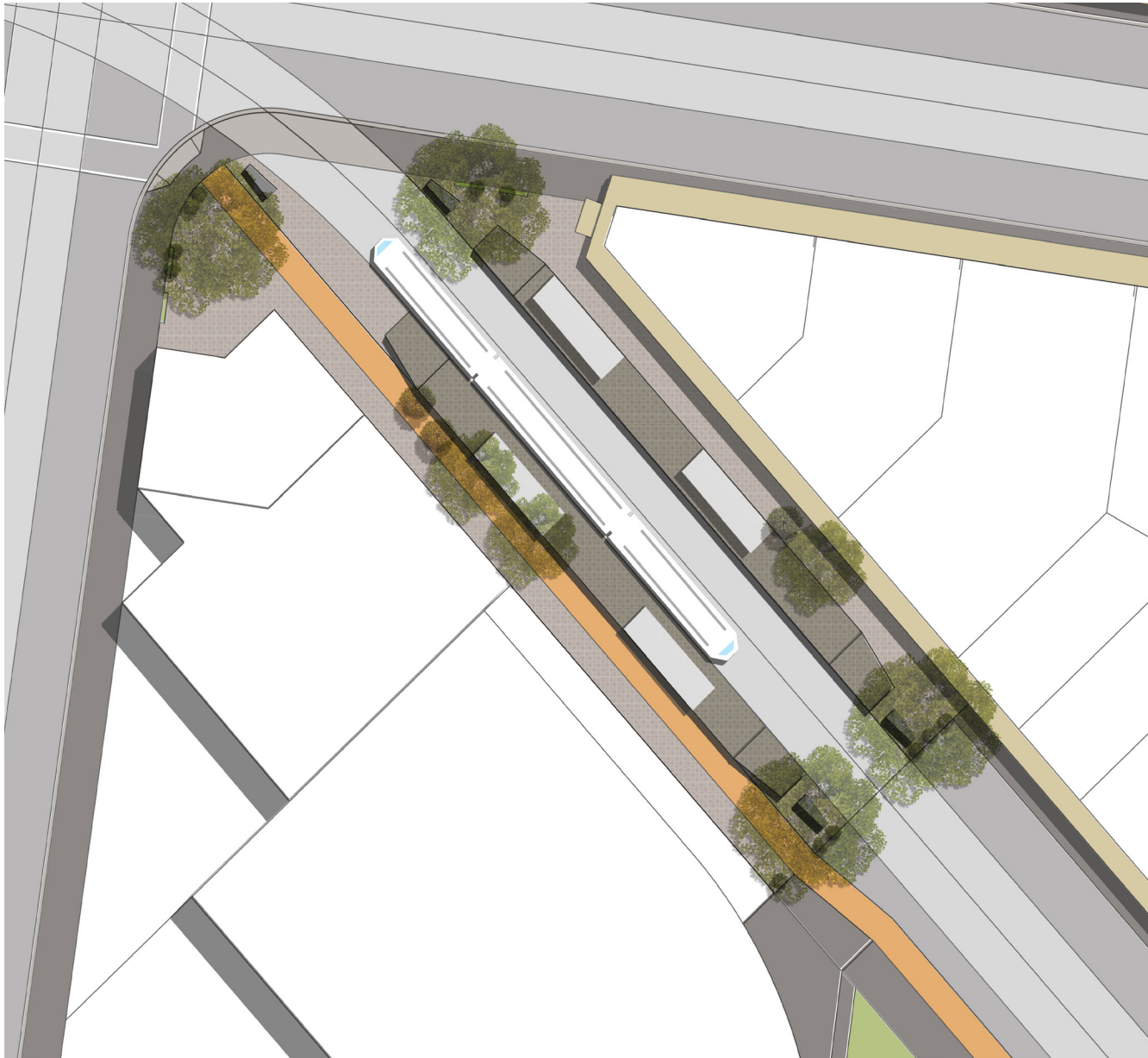
Figure 17: Indicative design of the southern plaza, showing the superstop for tram route 75.
